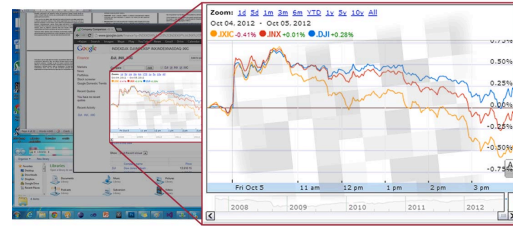
Figure 9. On a large desktop screen, a marker is mixed into the image for short periods of time so that a mobile device can reliably capture the exact location within the screen. Once the mobile device knows the location, the marker is displayed only in the vicinity of the mobile’s view frustum so that it is as unobtrusive as possible. If enough distinct and stable keypoints are present, the marker is completely hidden and camera the pose is tracked.
