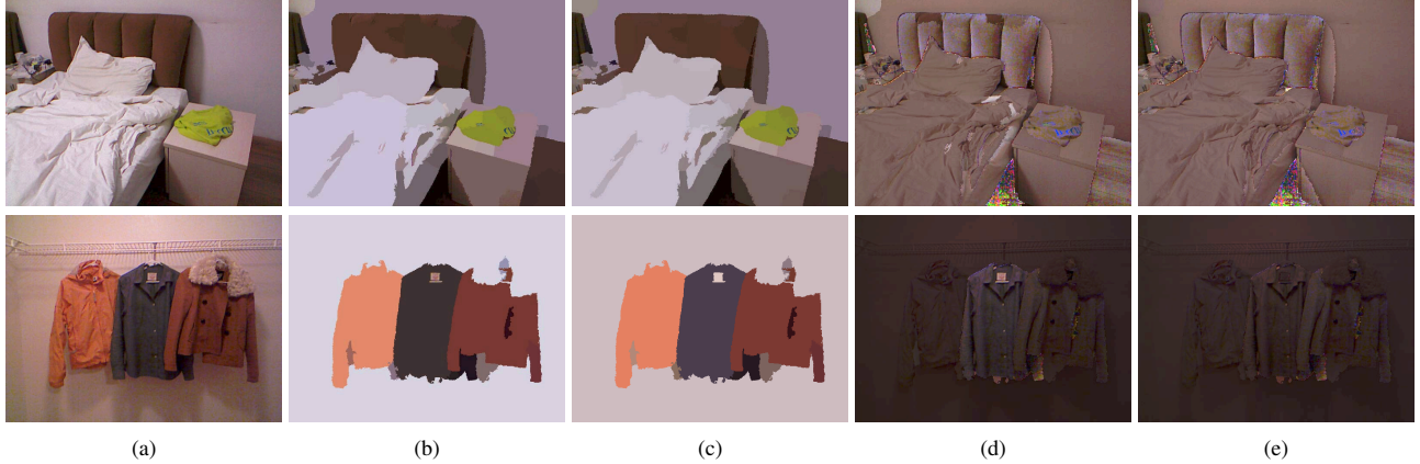
Figure 4. Relative albedos estimated by our alternating optimization. (a) Input image, (b) & (c) Relative albedos estimated at the 1st and 5th iteration, (d) & (e) Corresponding shading images at the 1st and 5th iteration. Clusters without relative albedos in the 1st iteration are simply filled by original RGB values in (b).
