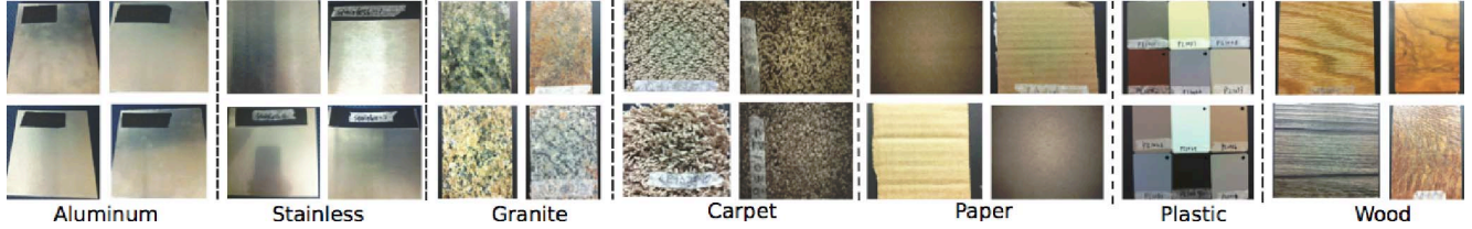
Figure 1: Samples in the spectral BTF database for material classification. The database includes eight classes of materials ( i.e. , aluminum, stainless, granite, carpet, paper, plastic and wood) and 90 samples in total. Each sample is imaged under 6 \times 25 = 150 lighting conditions (6 in wavelength and 25 in angular) with a resolution of 1040 \times 1392 . The database is available at http://compimg1.cis.rit.edu/data/texture/ .
