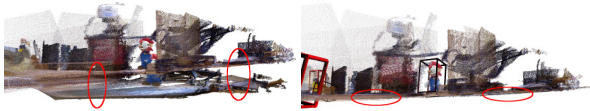
Figure 4: 7-objects sequence: without explicit loop closure detection a plain SLAM engine (left) accumulates error over time, whilst the ability to detect Mario allows our technique to also constrain the last and first frames and thus to tear down the global error (right).
