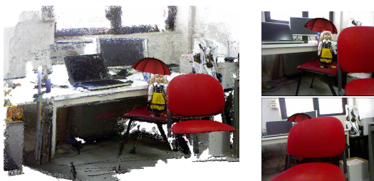
Figure 8: AR with 3D occlusion handling: once the Doll is detected (top right) a red umbrella can be rendered, even when the object is later occluded (bottom right); the final augmented 3D reconstruction is shown on the left.
