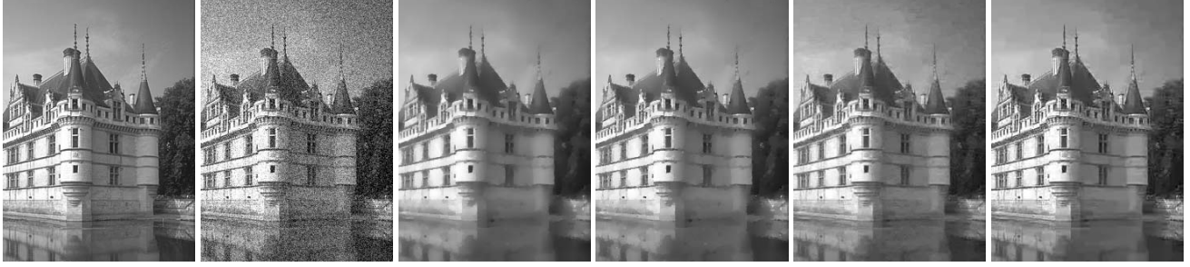
Figure 3. Natural image denoising problem. Displayed is the zoom into the right part of watercastle. Non-convex norms yield sharper discontinuities and show superiority with respect to their convex counterparts. From left to right: Original image, degraded image with Gaussian noise with \sigma = 25 . Denoising with TGVP prior, \alpha_1 = 0.5 , \alpha_2 = 1.0 , \lambda = 5 ( PSNR = 27.19 ), and non-convex log TGVP prior with \beta = 2 , \alpha_1 = 0.5 , \alpha_2 = 1.0 , \lambda = 10 ( PSNR = 27.87 ). The right pair compares the learned prior with convex norm ( PSNR = 28.46 ) with the learned prior with non-convex norm p = 1/2 ( PSNR = 29.21 ).
