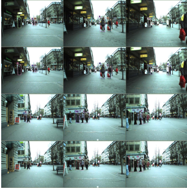
Figure 5: Rows 1 and 2 compare results of the dynamic programming (DP) algorithm of [13] and our algorithm respectively on the ETH sequence (frames 50, 90 and 106 shown). A pre-trained pedestrian tracker is used, and no occlusion handling is done for either algorithm. Rows 3 and 4 show tracking results using ground truth detections (frames 274, 304 and 319 shown). Row 3 shows the results from the DP algorithm, and row 4 shows our results. In this experiment, we allowed occlusion handling of up to 8 frames for both methods. The results show that our algorithm maintains ID labels more reliably.
