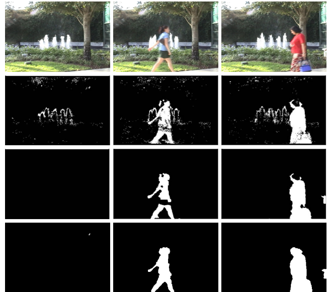
Figure 5: The top row are the original images from Fountain dataset [23]. The second row are the results obtained by using Bayesian modeling [23]. The third row are results obtained by the proposed method.
