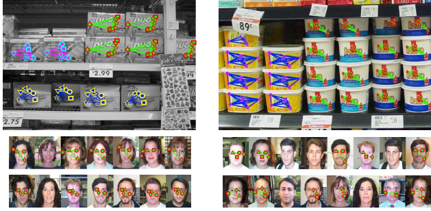
Figure 6. TOP: Sample results of our algorithm on the supermarket scene (Table 1) where it captures multiple recurring patterns in single images. BOTTOM: Sample results on a collage from the face dataset with object-level precision rate 98.4% and recall rate 63.8% (Table 1 right column).
