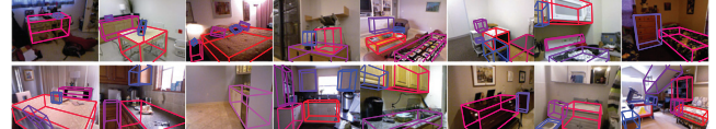
Figure 8. Sample images with ground truth cuboid labeling. The saliency of the labeled cuboids are denoted by the color: the warmer the color, the more salient the object is. There are 215 ground truth images and totally 476 labeled 3D cuboids.
