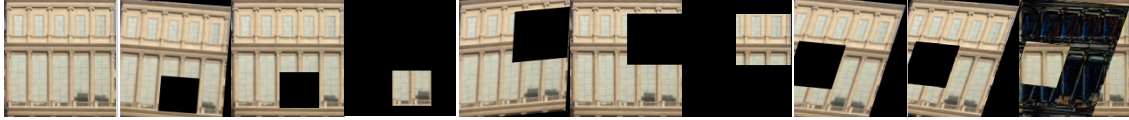
Figure 6. Qualitative results of the proposed single frame alignment method (Algorithm 2) with respect to translation, rotation, skew and occlusion. The first picture is the reference. Every three pictures of the rest are in one group, which represent the deformed and polluted version of the reference, the transformed result by our proposed and the corresponding residual, respectively.
