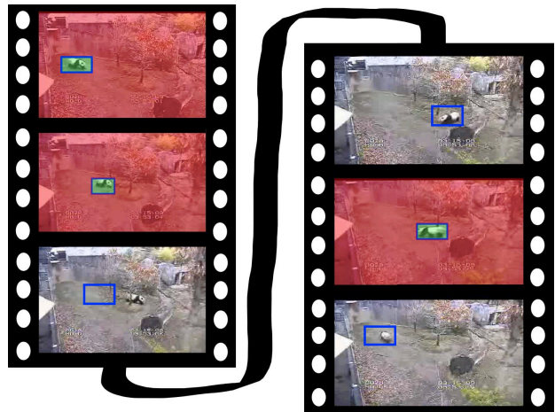
Figure 1. Our tracker uses self-paced learning to select reliable frames from which to extract additional training data as it progresses (shown in red). We use such frames to define both positive examples and a very-large set of negative examples (all windows that do not overlap each positive). By re-learning a model with this additional data, and re-tracking with that model, one can correct the errors shown above. We show that it is crucial to revisit old frames when adding training data; in terms of self-paced learning, a concept (frame) that initially looks hard may become easy in hindsight.
