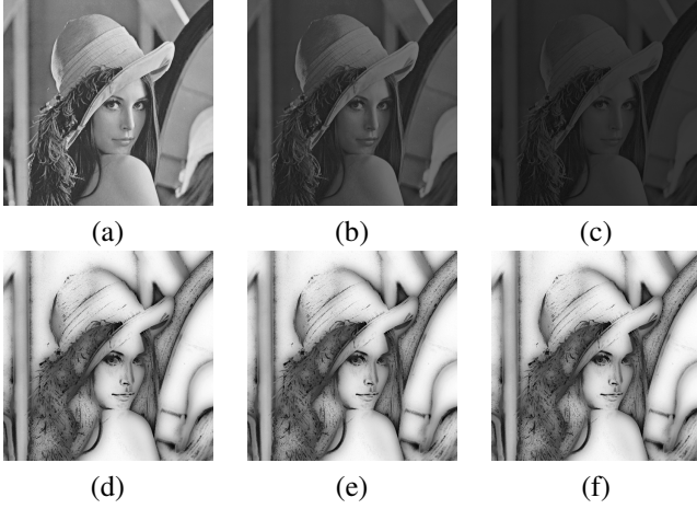
Figure 2: Illumination invariant features. (a)-(c) are input images with different illuminations. (d)-(f) are the corresponding outputs.
