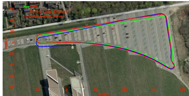
Figure 9. Trajectories before and after pose-graph loop-closure compared with GPS/INS ground truth.
