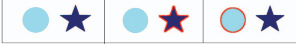
Figure 5. An example in which the curvature term affects our model’s output. The first image is the input image. The second image shows the output without curvature term. Last image shows the output using curvature term. (Better viewed in color.)
