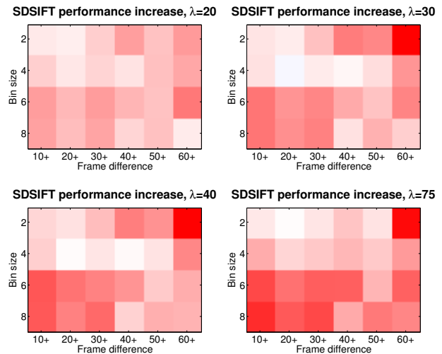
Figure 7. Increase in average overlap using our approach on DSIFT, from white (no difference in overlap) to red (largest increase in overlap, which is 0.14). For clarification, note the correspondence between the bottom left picture and Fig. 6 ( \lambda = 40 ).
