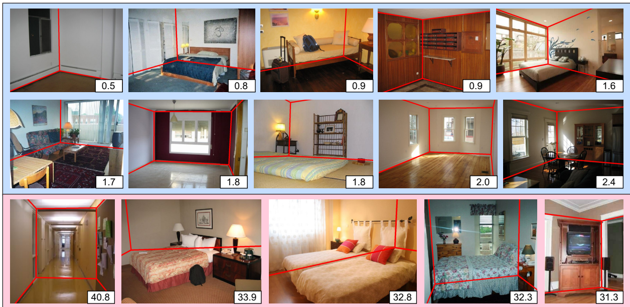
Figure 8. Layout estimation results on Hedau et al.'s dataset [9]. The 10 best (top) and 5 worst (bottom) results are shown with the pixel misclassification error percentages. Note the accuracy of the layouts despite using a coarse sampling. We obtain the high boundary accuracy because we detect not only visible junctions, but also occluded ones if there are line segments supporting them.
