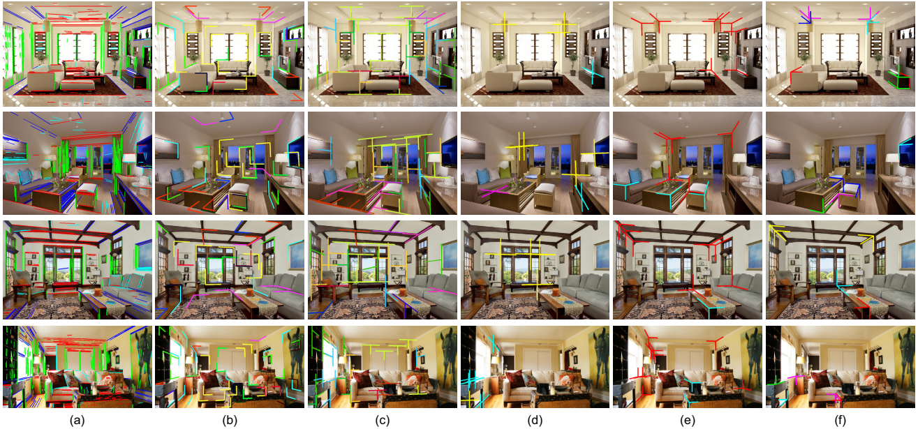
Figure 7. (a) Input images with detected line segments. (b–f) Detected junctions for each type of L, T, X, Y and W, respectively. For visualization purpose, only a subset of junctions that have the highest score in their small neighborhoods for each type are shown.
