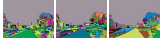
Figure 3: Video segmentation results by applying [10]. From left to right: Hierarchy levels in increasing order; region area increases as segments from lower hierarchy levels are grouped together.
