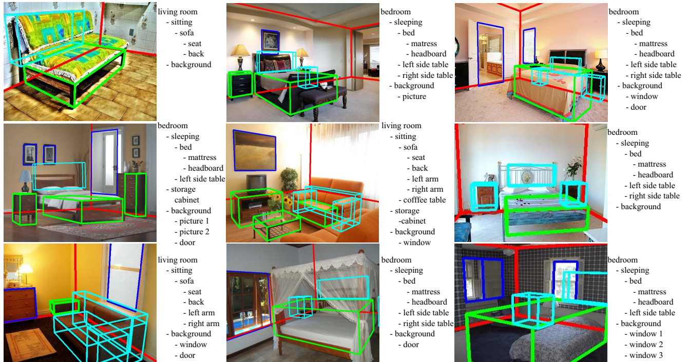
Figure 7. Parsing results include cubic objects (green cuboids are detected by bottom-up step, and cyan cuboids are detected by top-down prediction), planar objects (blue rectangles), background layout (red box). The parse tree is shown to the right of each image.
