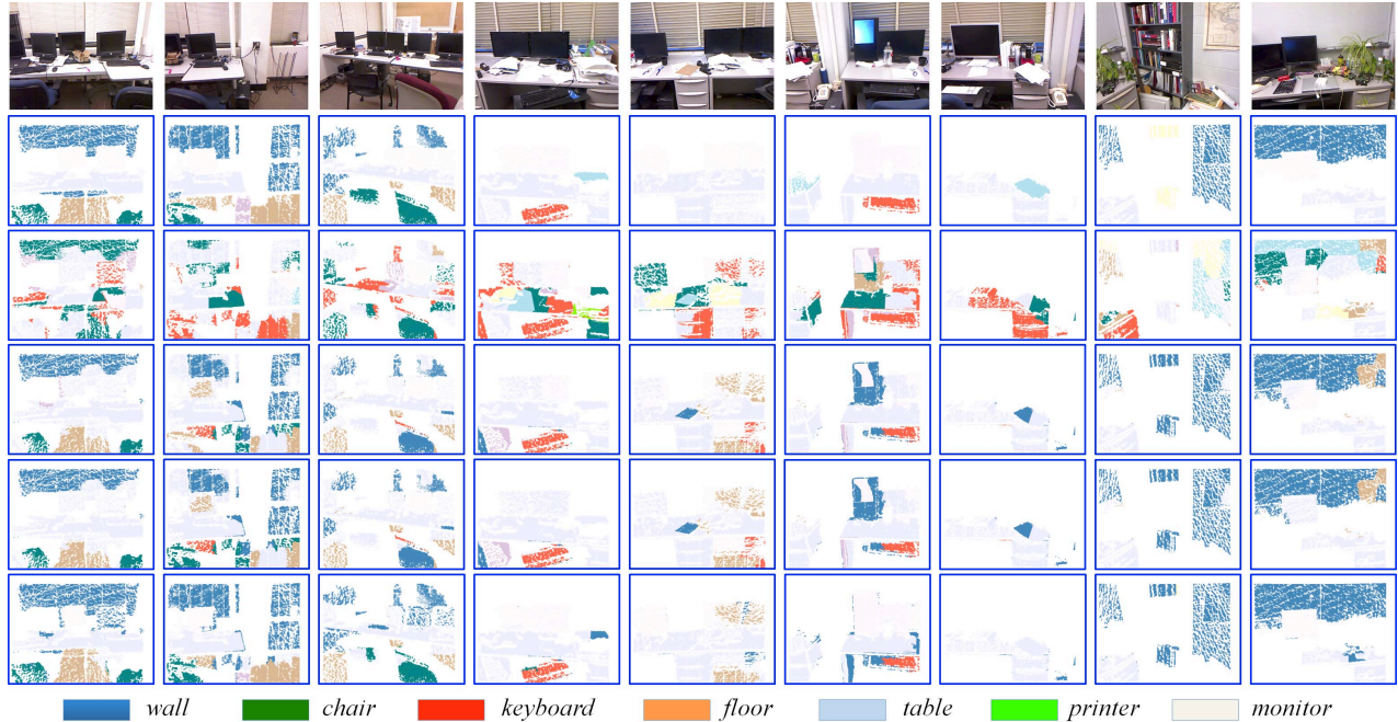
Figure 5. Example results of point cloud labeling on Cornell dataset [16]. To demonstrate labeling results with more details, reference images from multiple views are provided. The rows are, reference images, ground truth, labeling result from Naive k NN, ESVM, ESVM with refinement, and our oracle performance.
