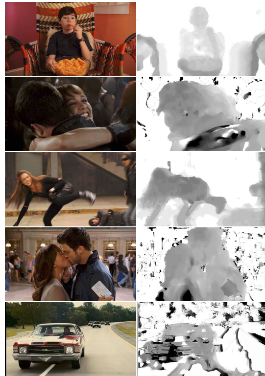
Figure 1: Example frames of various action sequences from the dataset, showing the left viewpoint and depth streams. Darker regions of the depth image are closer to the camera. From top to bottom the actions are Eat , Hug , Kick , Kiss and Drive .
