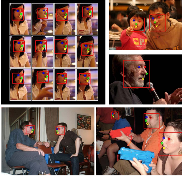
Figure 8. Examples of face alignment. The landmarks are accurately localized in different conditions.
