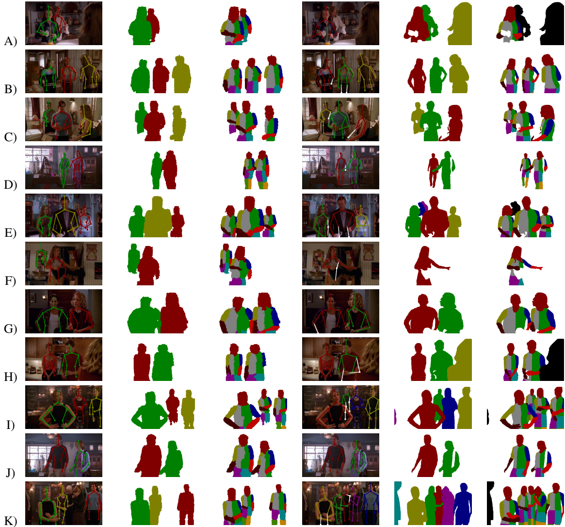
Figure 3. Qualitative results on the Buffy data set. The first three columns are the pictorial structure pose, instance segmentation and body-part segmentation obtained using our method; the last three columns are the corresponding ground truth. The method can naturally handle multiple instances. The algorithm successfully estimated the large majority of the instances and the locations of their joints. Furthermore, there are examples of partial occlusion by another person (A right, C left), a background object (C left) and self-occlusion (B right, C right). Some of the images also demonstrate failings, including: a phantom hallucinated instance (F left), a missed part in an uncommon location (F right), incorrect visibility of the part (B right, H right), limb assigned to a wrong person (D left / right), a missed instance due to a large occlusion (I middle) or an insufficient number of candidates for images with too many instances (K middle).
