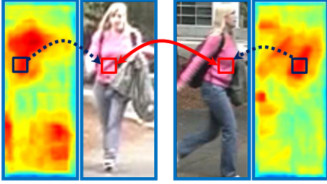
Figure 5. Illustration of bi-directional weighting for patch matching. Patches in red boxes are matched in dense correspondence with the guidance of corresponding saliency scores in dark blue boxes.
