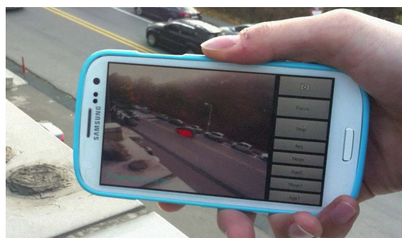
Figure 1. Example of the proposed method running on a mobile device (foreground pixels highlighted in red). Our implementation runs approximately 20 frames per second, comfortably in realtime.
