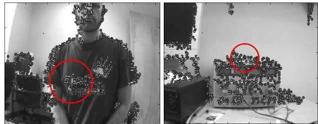
Figure 6: Collision estimations provided by the portable embedded prototype. Red circles identify the colliding objects for a static camera scenario, where a person is approaching the camera plane with a head-on trajectory (Left), and moving camera in a collision trajectory with surrounding objects (Right).
