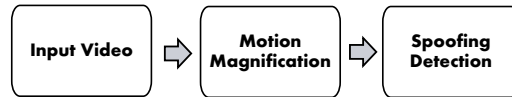
Figure 2. Motion magnification of input video may accentuate facial expressions thereby aiding spoofing detection techniques.
