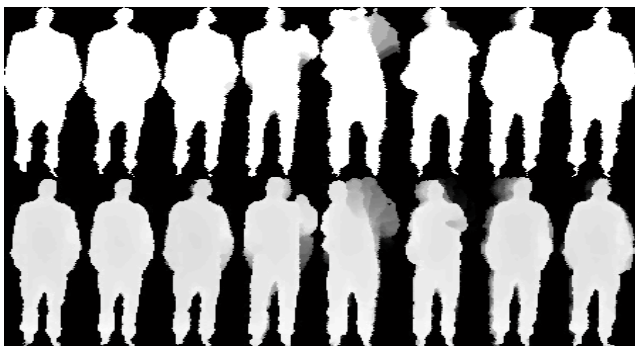
Figure 2: A comparison of MHI (top) with MDI (bottom). MDI tracks the motion of depth changes.
