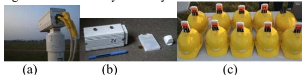
Figure 1. (a) Shows a UWB receiver deployed in the field (b) shows the asset tracking system components, ultra-wideband radio frequency receiver (shown with integrated high-gain antenna), 1 W transmitter tag, and 30 mW transmitter tag. c) Several tags are shown attached to helmets to track people in a scene.
