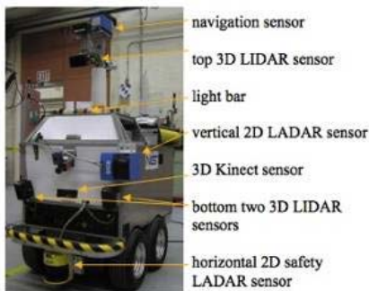
Figure 6a. AGV with various onboard sensors.
