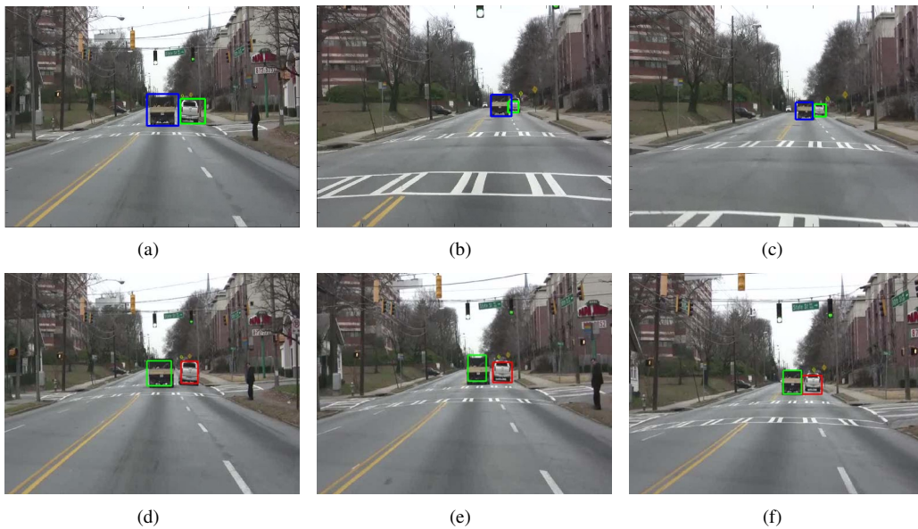
Figure 5. Experiment 2 Detection: (a) frame 16, (b) frame 94, (c) frame 115; Tracking: (d) frame 9, (e) frame 31, (f) frame 51.
