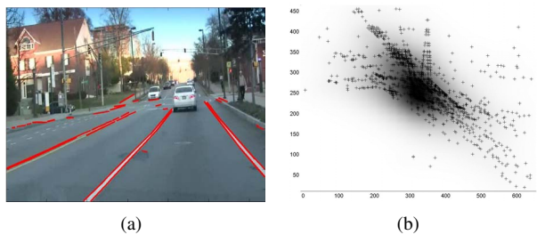
Figure 2. Horizon detection (a) lines around the boundary of superpixels that are close to the bottom FOV, (b) density of intersections
