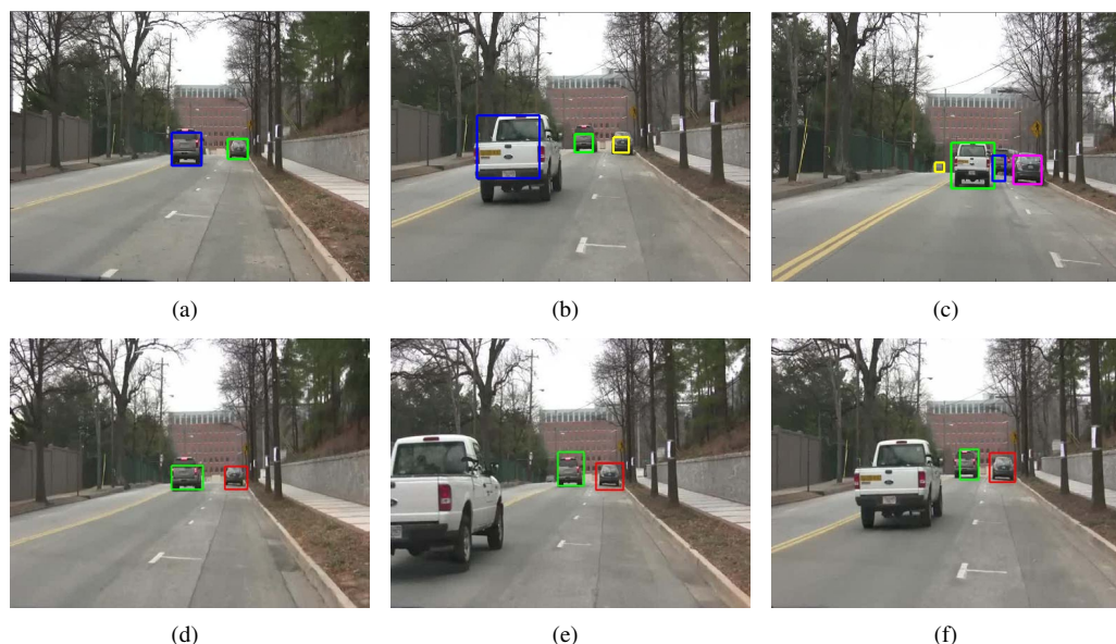
Figure 6. Experiment 3 Detection: (a) frame 123, (b) frame 177, (c) frame 213; Tracking: (d) frame 126, (e) frame 153, (f) frame 171.
