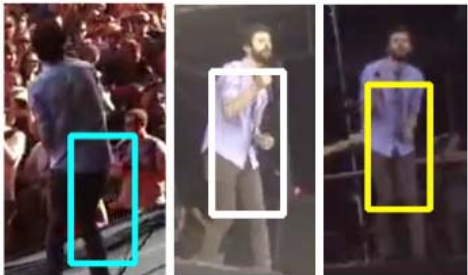
Figure 7. Three simultaneous views of a selected subject. The subject is tracked in Camera B using the MIL tracker (center), and the track box is projected into two other views (left and right).
