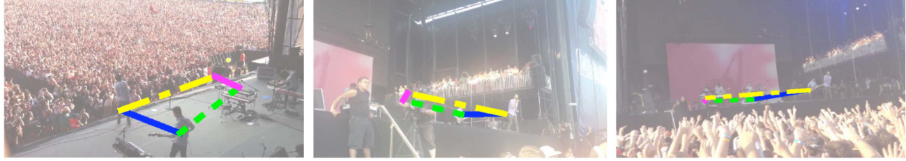
Figure 8. A plane drawn in Camera A (left) of our test sequence is reprojected accurately in Camera B (center) and Camera C (right).
