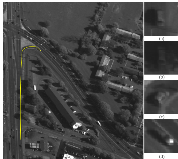
Figure 1. A typical path of a car in CLIF data is marked in yellow on the image in left. Images (a), (b), (c) and (d) show the variation in views of the same car when it traverses the path marked in yellow.
