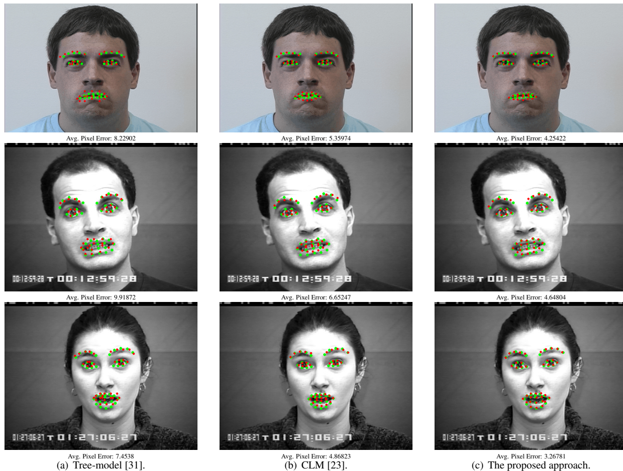
Figure 8. Qualitative comparison of Tree-model [31], CLM [23] and the proposed approach (best viewed in color and high-resolution, green: ground truth, red: algorithm-specific results, less green seen means a better fit).
