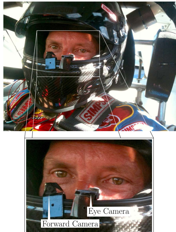
Figure 1. Early prototype for initial data collection in a NASCAR race circuit. This prototype consists of a forward facing camera to observe the environment from the driver’s point of view and an eye facing camera for estimation of the gaze direction. Both cameras are connected to a laptop computer for data recording.
