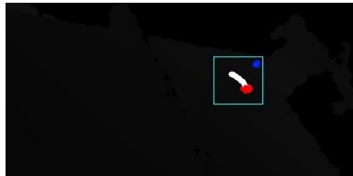
Figure 6. Detection of ball candidates in a depth image. White curve is 2D trajectory reconstructed based on RGB images. Rectangle is the range of positions where ball can be, which was defined with the trajectory. Red segment was selected as ball, and blue segment was rejected.
