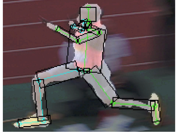
Figure 5. Image with mask overlay and keyframe skeleton with part regions that part models are built from.
