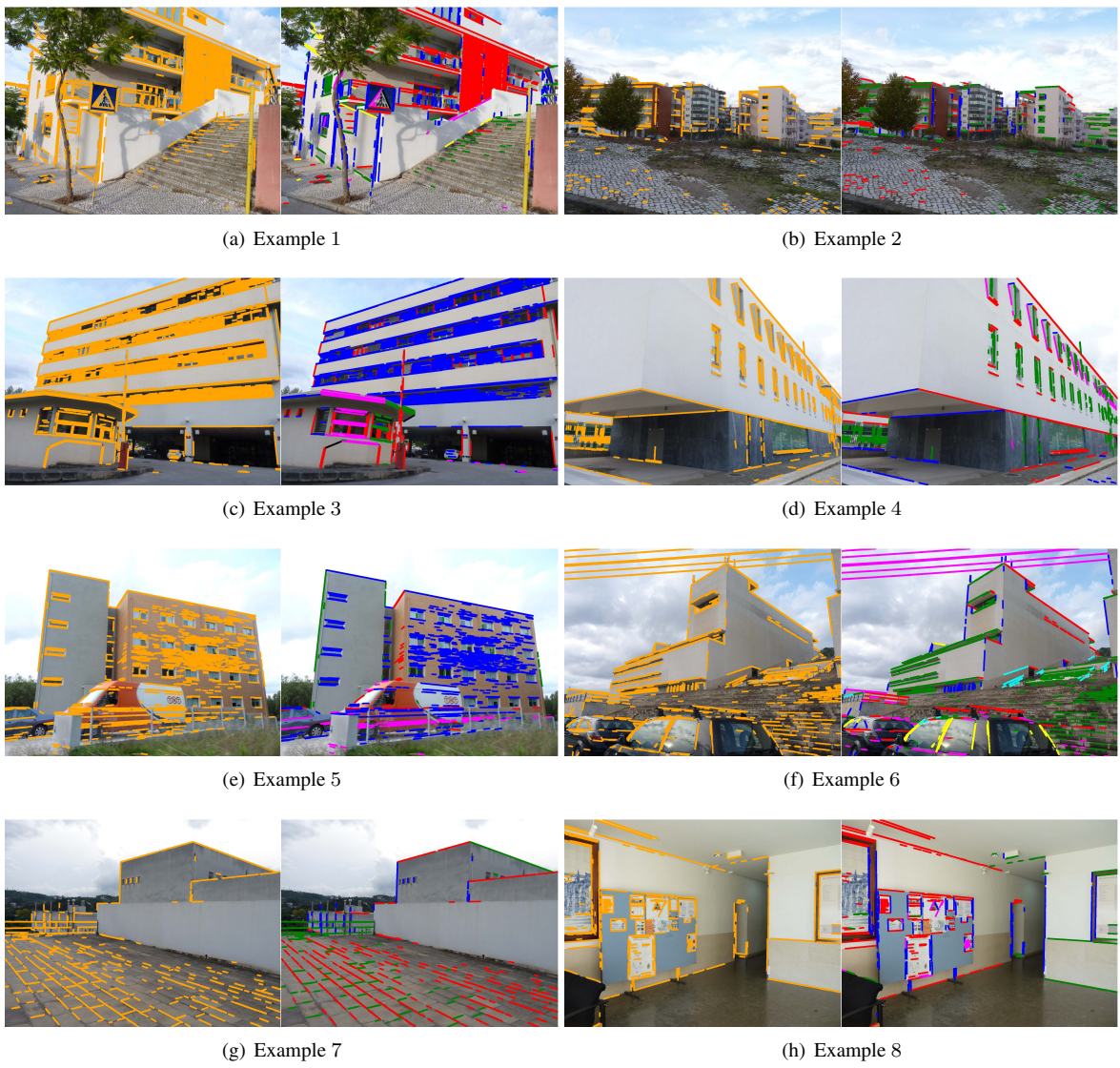
Figure 3. We show 8 examples from our dataset. The left images show the input edges (orange), while the right images show the clustering results. We detect the VDs of the Manhattan world (red, green and blue), VPs that are non-orthogonal to the Manhattan triplet (yellow, magenta and cyan), and lines that are considered outliers (black, no VP is assigned). This is performed simultaneously by our algorithm.
