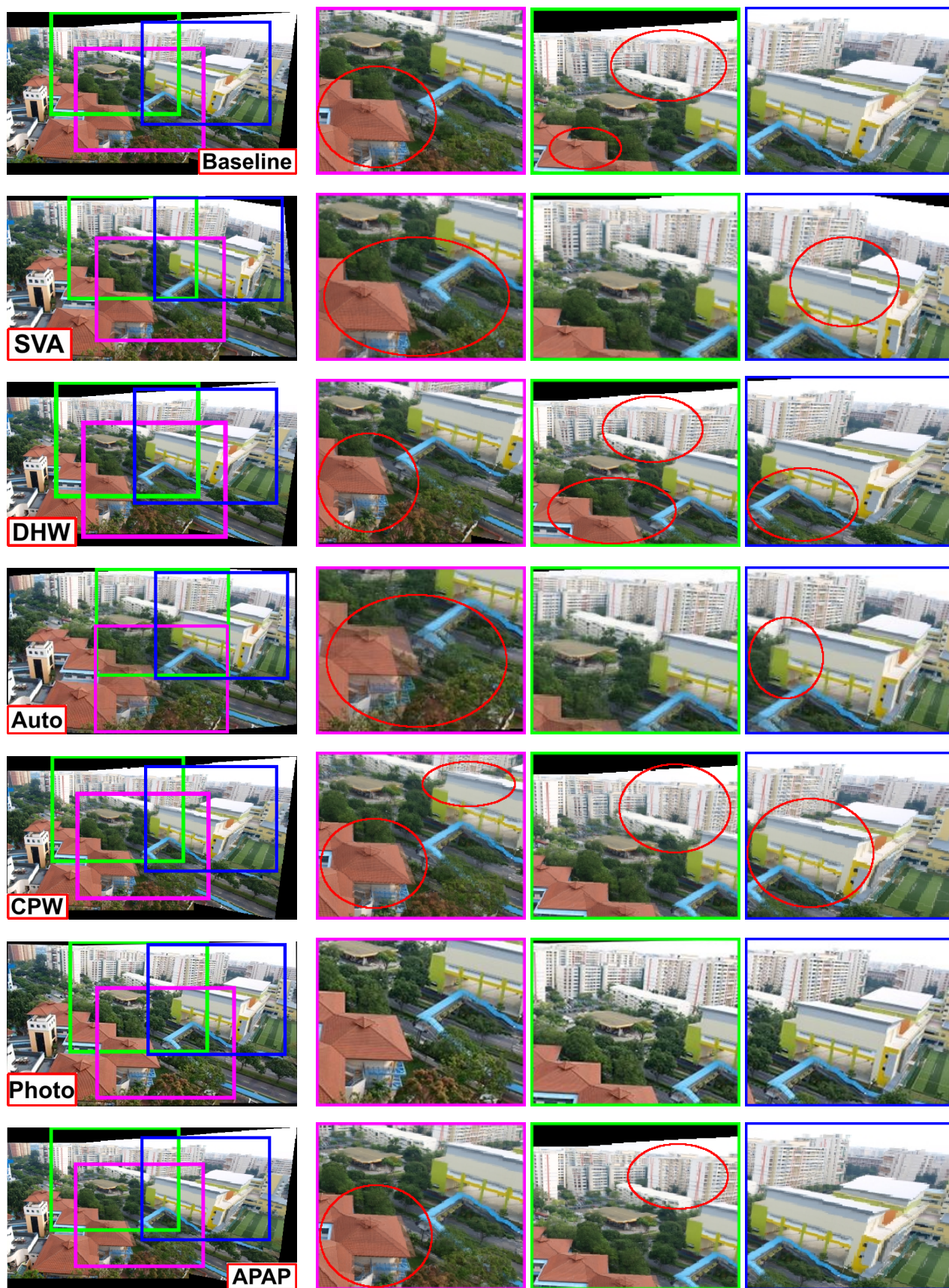
Figure 9: Qualitative comparisons (best viewed on screen) on the rooftops image pair. Red circles highlight errors. List of acronyms and initialisms: SVA-Smoothly Varying Affine, DHW-Dual Homography Warps, Auto-Autostitch, CPW-Content Preserving Warps, Photo-Photosynth, APAP-As Projective As Possible Warps.
