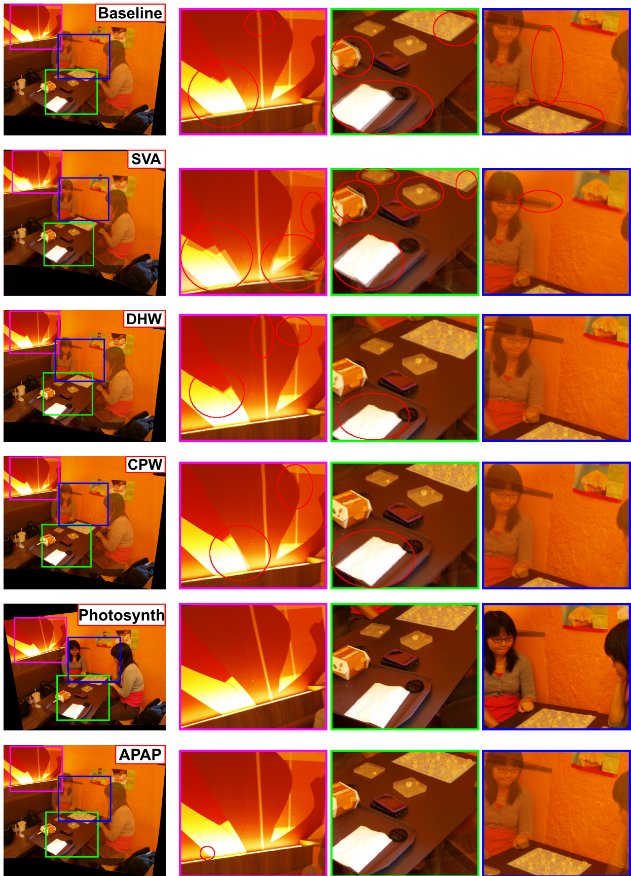
Figure 7: Qualitative comparisons (best viewed on screen) on the chess/girl image pair. Red circles highlight errors. List of acronyms and initialisms: SVA-Smoothly Varying Affine, DHW-Dual Homography Warps, CPW-Content Preserving Warps, APAP-As Projective As Possible Warps.
