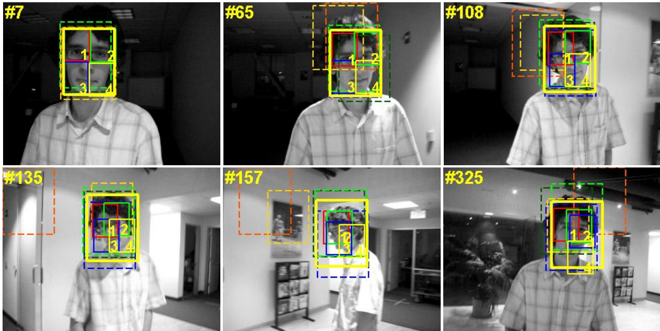
Figure 3. Qualitative visual tracking results of our tracker and competing trackers over representative frames of board sequence. Note that the number marked on small rectangles represents the index of object parts.
