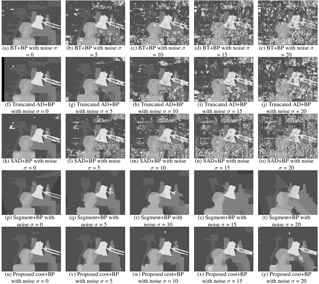
Figure 5. Results of test stereo algorithms on noisy Tsukuba image pair with varying standard deviation of noise \sigma .
