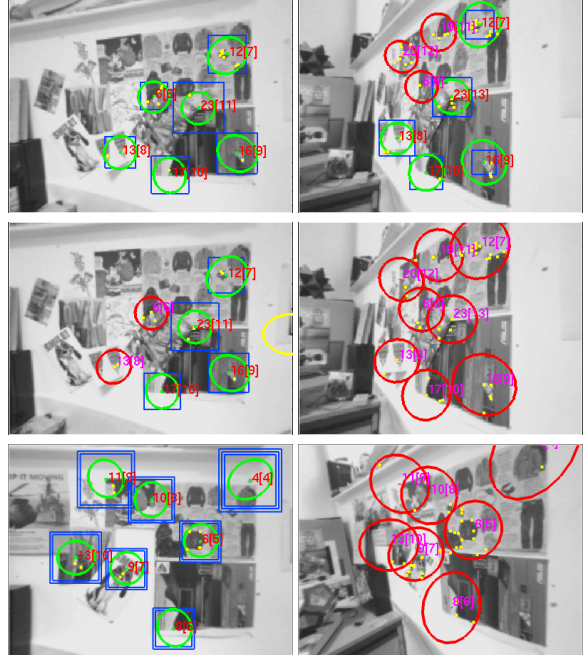
Figure 4. Feature matching performance during SLAM, comparison between the new method and that in [1] : (top) new method; (middle) new method without exemplars; (bottom) method in [1].
