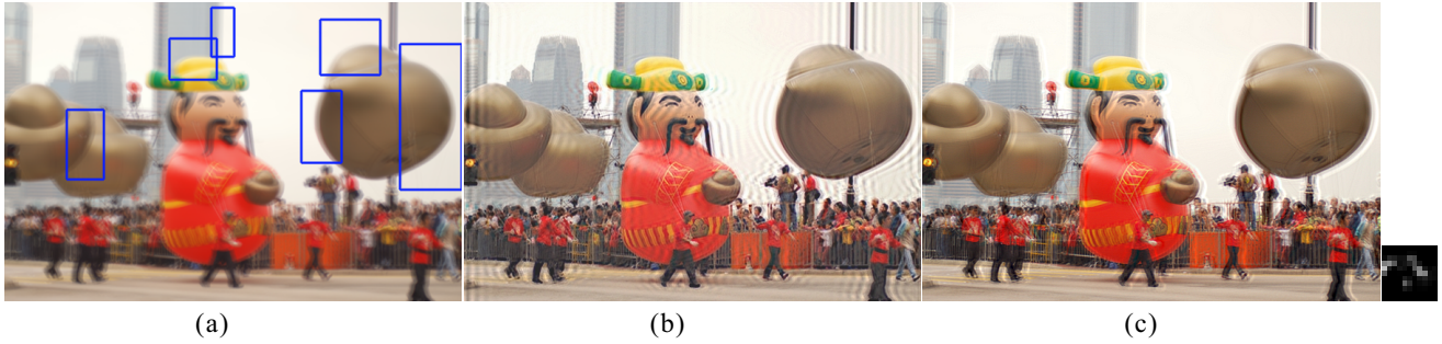
Figure 10. Example of camera motion blur. (a) The input blurred image. Patches are selected within the blue rectangles where the transparency values are computed. (b) The deblurred image from the method in [21]. (c) The deblurred image using our estimated blur filter shown on the right.
