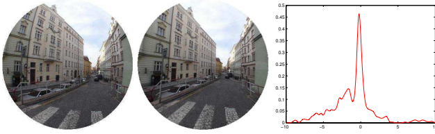
Figure 6. Real data. (Left) Input image with significant radial distortion. (Center) Corrected image. (Right) Distribution of real roots obtained by kernel voting for this image and estimated \lambda = -0.22 .
