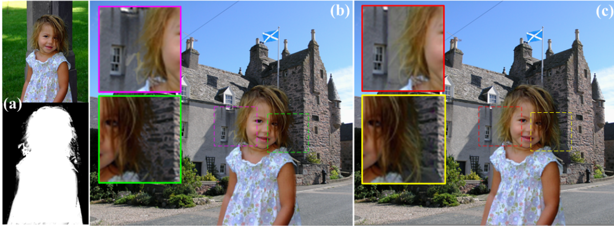
Figure 9. (a). Original image and matte extracted by Bayesian matting. (b). Composition created by Bayesian matting. (c). Composition created by our algorithm.
