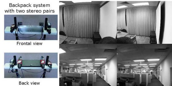
Figure 1. Front and back views of the backpack system and sample images captured as the person enters a room.
