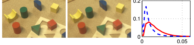
Figure 5. Edge significance PDF. Left: Input image, Centre: Image blurred with a Gaussian ( \sigma = 1.2 ). Right: PDFs for the edge significance measure. Solid curve is the PDF for the original image, dashed curve is the PDF after Gaussian blur.
