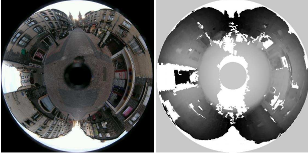
Figure 4. Reference image 211 and its depth map (white pixels have no depth).
