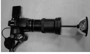
Figure 1. The “0-360” mirror with the Nikon Coolpix 8700.
