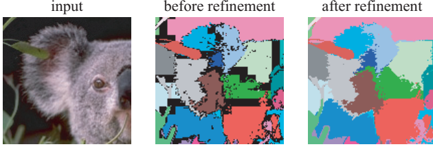
Figure 5. After mode extraction, most pixels are segmented, only boundaries remain unclassified (black pixels in middle image). These pixels are clustered using an iterative process that stops as soon as it reaches a labelled region (result shown on the right).
