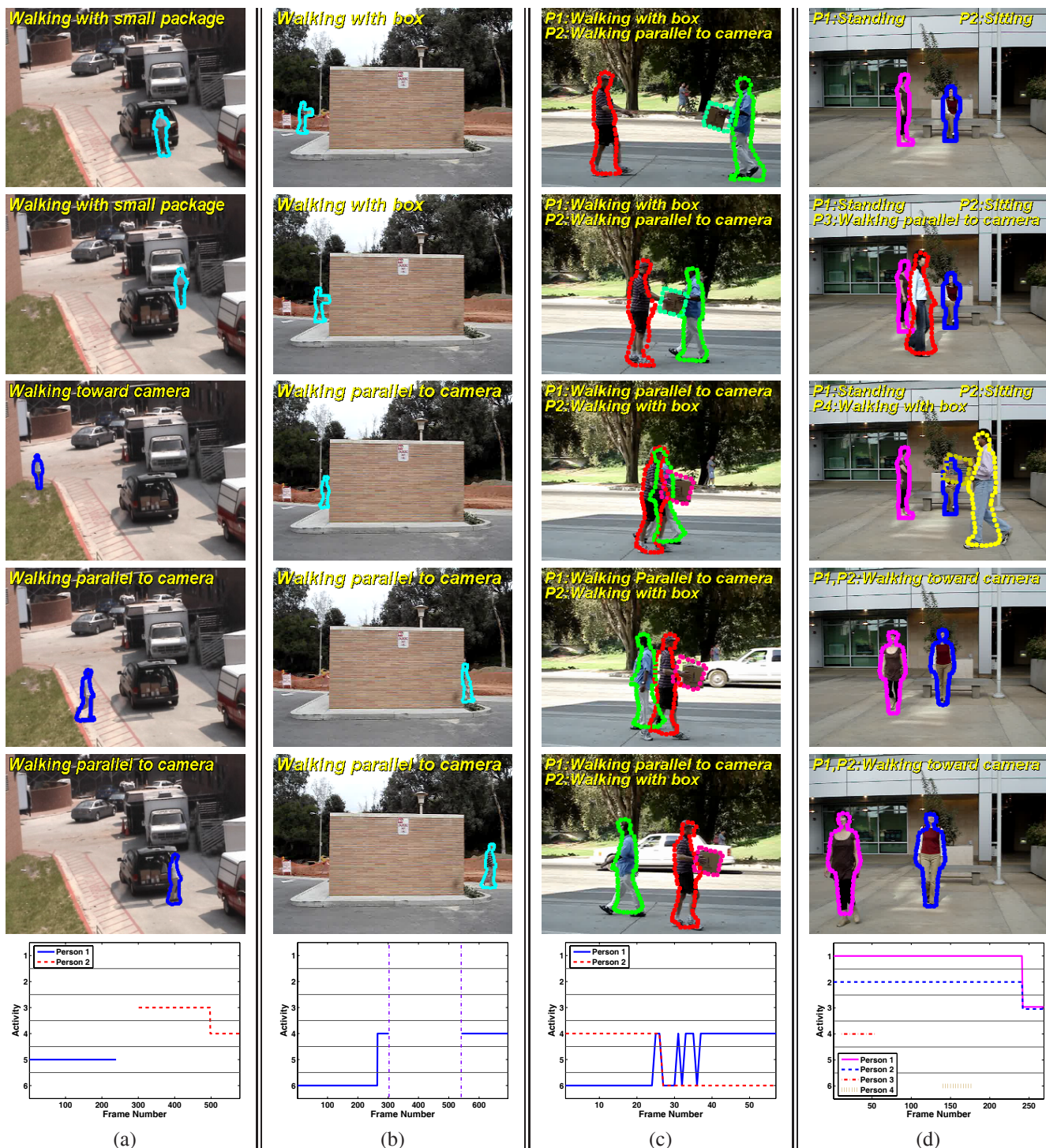
Figure 7. Row 1-5: Tracking results with the activity models used to track shown on the top. Row 6: Model switching results. The labels denote: 1: Standing, 2: Sitting, 3: Walking toward camera, 4: Walking parallel to camera, 5: Walking with small package, 6: Walking with box. (a): Tracking results on an outdoor sequence. (b): A person walking with a box, disappearing behind a wall, and emerging on the other side without the box. We do not track when the person disappears behind the wall. Tracking restarts when we detect that the person has reappeared; (c): Two person walking towards each other, one person holding a box then giving it to the other person. At the first frame, the activity of person 1 is initialized as “walking with a box”, then we split box from person and track them separately. (d): Multiple people doing different activities simultaneously. (The figure is best viewed on a monitor.)
