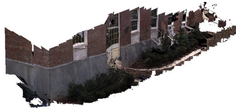
Figure 7. The reconstruction produced by our algorithm from several hundred frames of video. By testing only plane hypotheses with high prior probability, the reconstruction was achieved with only 48 plane hypotheses per frame at a speed of 20.0 Hz.
