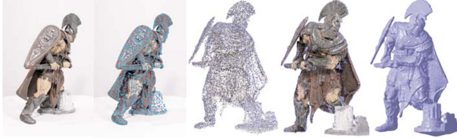
Figure 1. Overall approach. From left to right: a sample input image; detected features; reconstructed patches after the initial matching; final patches after expansion and filtering; polygonal surface extracted from reconstructed patches.
