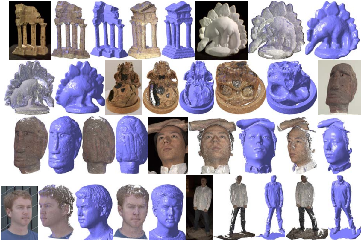
Figure 7. Sample results on object datasets: From left to right and top to bottom: temple , dino , skull , polynesian , face , face-2 , and body datasets. In each case, one of the input image is shown, along with two views of texture-mapped reconstructed patches and shaded polygonal surfaces.
